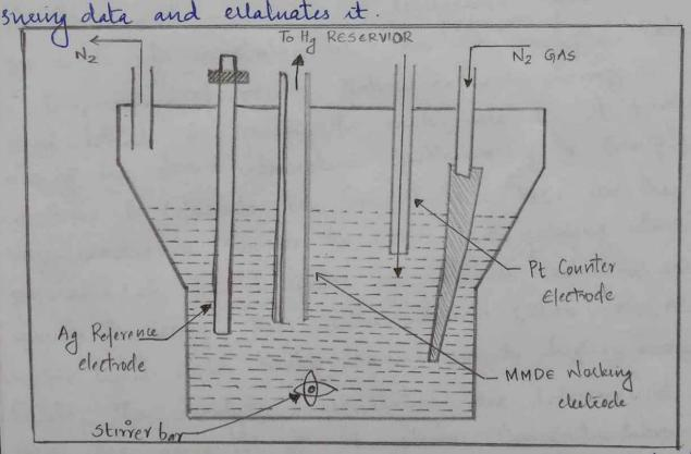
Computare Consist of 3 electrocle Byslem: Working dectrocke (Hg, Pt, Au, Ag), Reference electrode (SEE/ tg/tgcl) and Auxillary electrode (Pt wire, C). A potential is applied to an dectro chemical cell and the amount flowing through the cell is measured as a function of that potential. Various Applications of this
