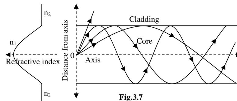
parabolic manner from maximum value at the centre of the core (axis of the fiber) to a constant value at the core-cladding interface. Since the refractive index of the core decreases as one move away from the axis, the rays entering into the fiber are continuously bent towards the axis of the fiber and the ray paths inside the fiber are sinusoidal. From the figure it is clear that light waves with large angles of incidence travel more distance than those with smaller angles. But the
