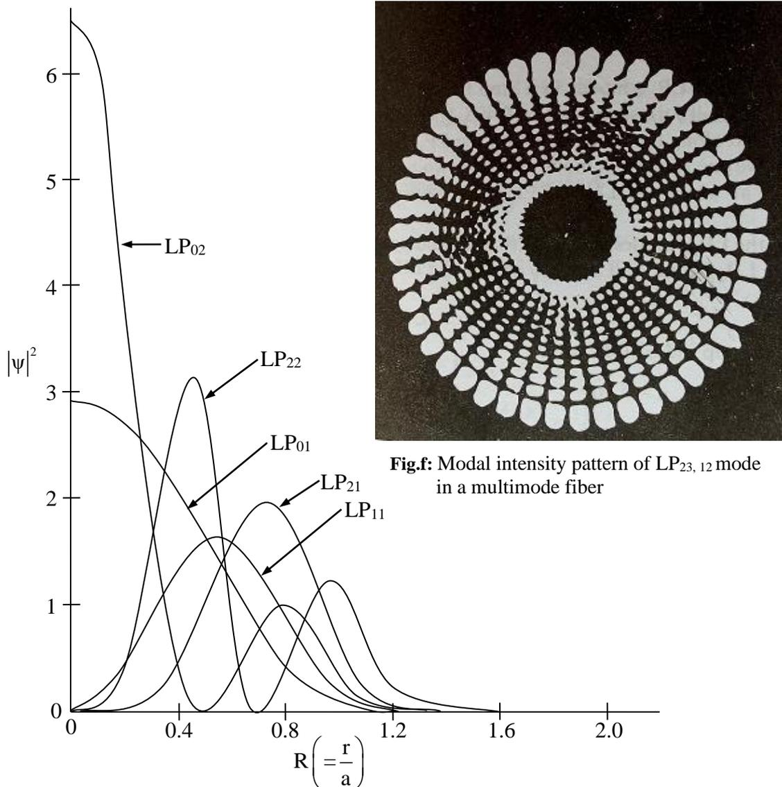
**Fig.d:** Radial intensity distributions of some low order modes in a step index fiber for  $V = 8$
