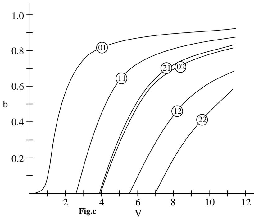
The condition  $b = 0$  (i.e. by eqn.19,  $\beta^2 = k_0^2 n_2^2$ ) corresponds to what is known as the cut off of the mode. For  $b < 0$ ,  $\beta^2 < k_0^2 n_2^2$  and the fields are oscillatory even in the cladding and the modes are known as radiation modes. At cut off,  $b = 0$ , by eqn.19,  $W = 0$  and by eqn.20,  $U = V = V_c$ .
